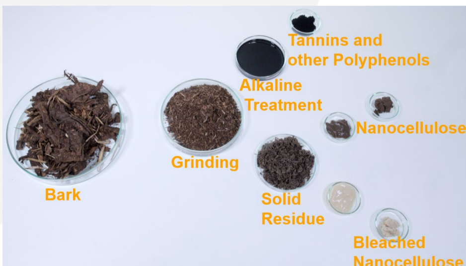
Fig. 2: Tannins are obtained through alkaline treatment and spray-drying; the remaining residues are further processed into nanocellulose
