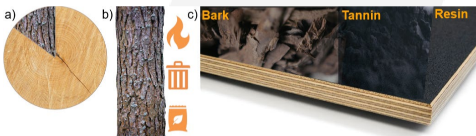
Fig. 1: a) Around 15% of a tree consists of bark, b) it is currently mainly burned, disposed of, or used only for low-value applications, c) however, valuable tannins can be extracted from bark, which can serve as the basis for a 100% biobased resin.
