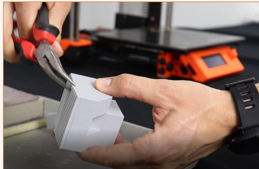
Using pliers for removing support structures. Source: CETEM
