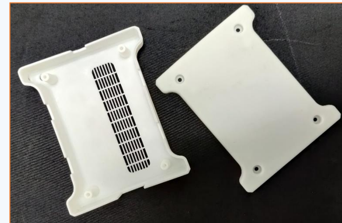
SLA printed prototypes. Proof of concept prototype Source: CETEM
