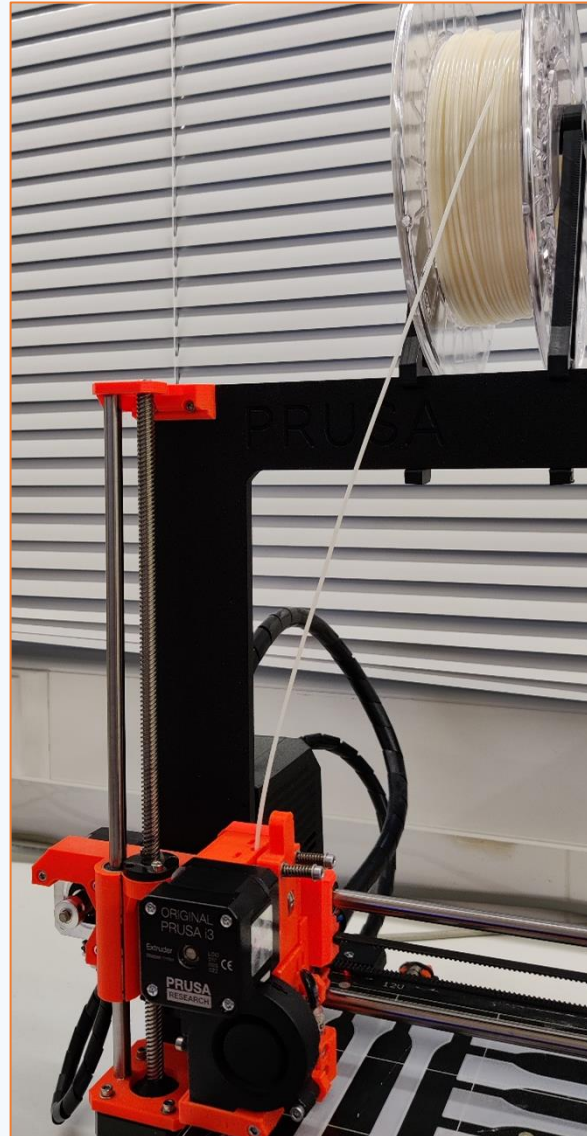
FDM machine. Detail of material feeding. Source: CETEM
