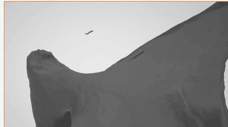
Some noise to eliminate in a 3D scanned model. Source: CETEM
