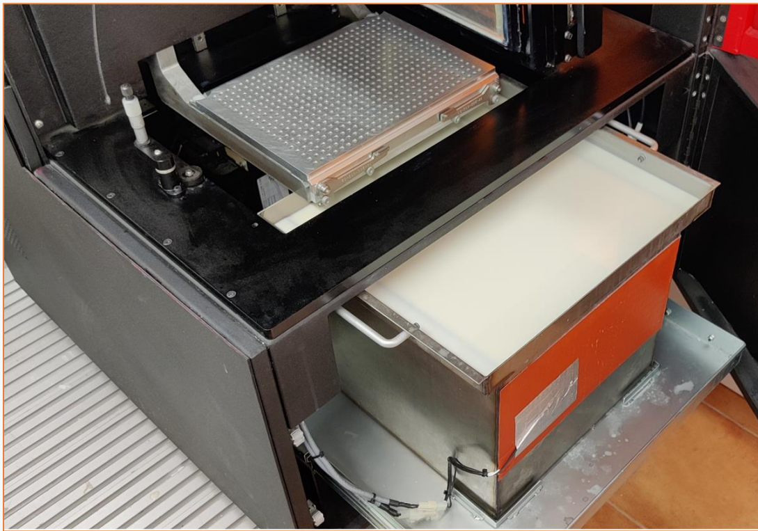
SLA machine. Detail of the bed or platform and the resin vat . Source: CETEM
