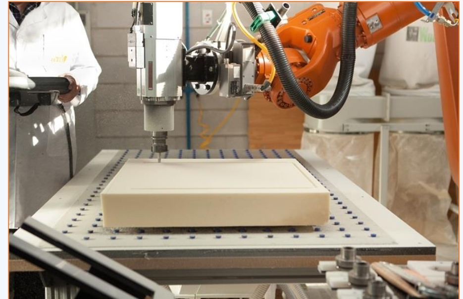
CNC machining. Source: CETEM.
